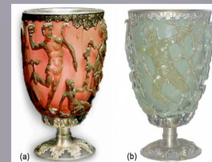
The cup of Lycurgus (nanostructured glass)
