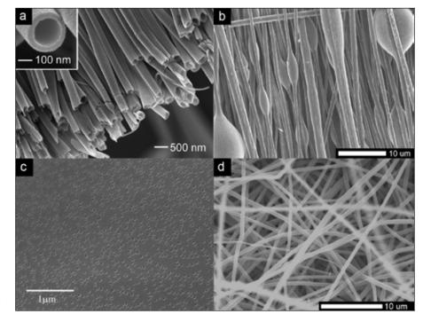
Fig. 3: (a) Hollow, aligned electrospun fibers; (b) Beaded, aligned polystyrene fibers; (c) Porous surface of a polystyrene fiber; and (d) Random mesh of TiO<sub>2</sub> fibers. (a) and (c) reprinted with permission from References 21 and 30, respectively. Copyrights 2004 and 2002, American Chemical Society.
