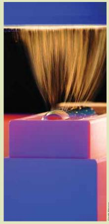
Elmarco's Nanospider nozzleless process can allow a large number of jets to form naturally out of a thin film of a polymer solution.
