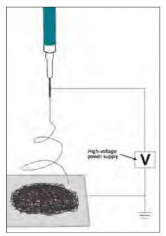
Fig. 2: Typical laboratory-scale electrospinning apparatus that allows production of milligram to gram amounts of ceramic nanofibers.
