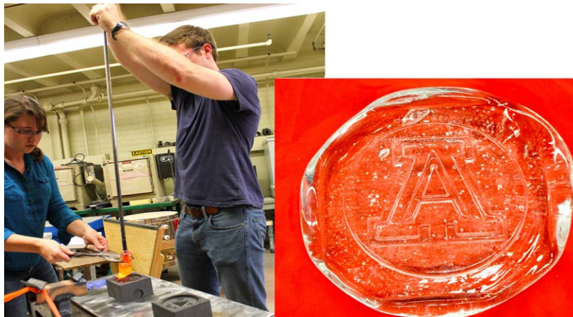
Figure 1: Student demonstrating glass molding of the wildcat A.
