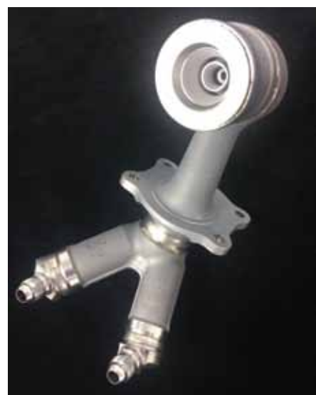
Figure 3. Cobalt-chromium fuel nozzle for GE's LEAP engine.
