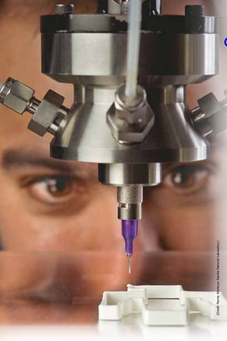
Figure 1. Robocasting deposits ceramic-loaded slurry through a syringe according to a computer-controlled pattern under the watchful eye of Joseph Cesarano.
