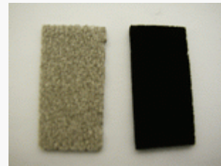
Co-B catalyst coated on Ni foam
