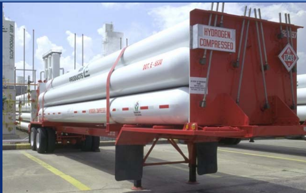
Gas Tube Trailer
