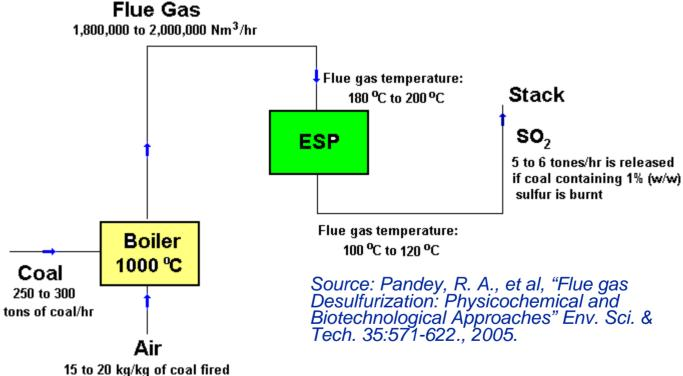
Generation of SO<sub>2</sub> in 500 MW coal fired power plants can produce huge amounts of SO<sub>2</sub> that can be used for the production of H<sub>2</sub> as well as fertilizers.
