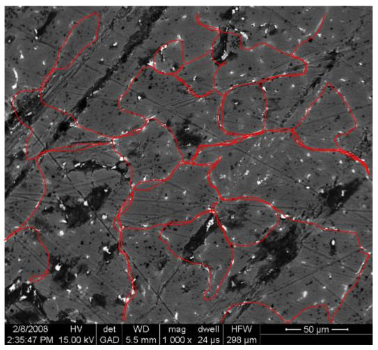
EDX image of 95 wt.% aluminum sample. Brighter regions indicate elements of larger atomic number (Ga, In, Sn). Phase segregation and grain boundaries can be seen.
