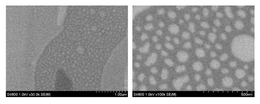
SEM image of what is believed to be a grain boundary of Ga-In-Sn containing AI nanoparticles
