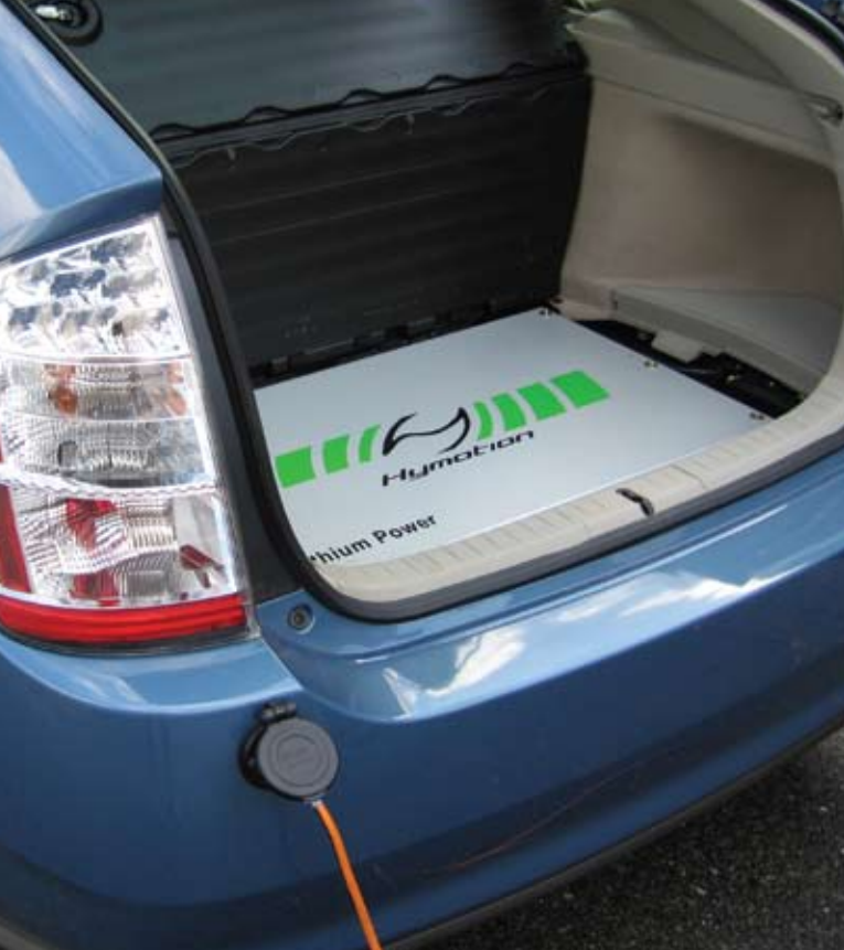
Thin packs can convert standard hybrid automobiles into plug-in vehicles. Achieve over 100 miles per gallon of gasoline
