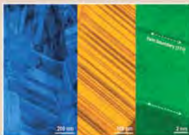
Nanostructured twin copper with ultra-high strength and high electrical conductivity.
