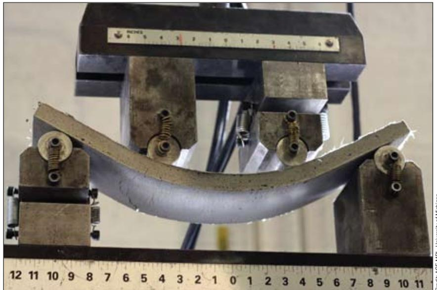
**Self-healing concrete works because it can bend. When it’s strained, many microcracks form instead of one large crack that causes it to fail. Here, a specimen is bending as a force of 5 percent tensile strain is being applied. Regular concrete would fail at 0.01 percent tensile strain.**
