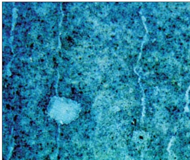
These close-up photographs illustrate how the concrete cracks (left) before and (right) after healing.
