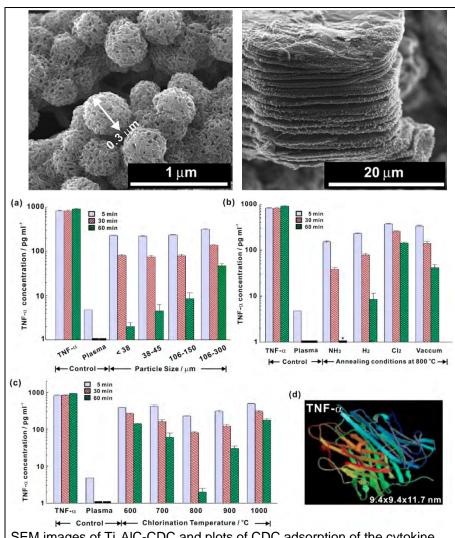
SEM images of Ti<sub>2</sub>AIC-CDC and plots of CDC adsorption of the cytokine TNF- $\alpha$  from human plasma as a function of (a) CDC particle size, (b) annealing gas, (c) chlorination temperature; (d) a model of TNF- $\alpha$ .
