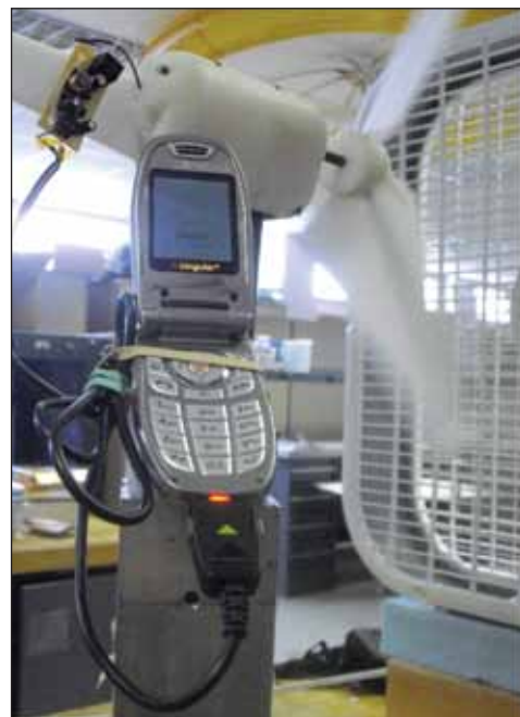
Fig. 7 Photograph a cell phone connected to the electrical charging circuit of the windmill.
