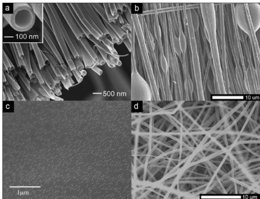
**Fig. 3:** (a) Hollow, aligned electrospun fibers; (b) Beaded, aligned polystyrene fibers; (c) Porous surface of a polystyrene fiber; and (d) Random mesh of TiO<sub>2</sub> fibers. (a) and (c) reprinted with permission from References 21 and 30, respectively. Copyrights 2004 and 2002, American Chemical Society.
