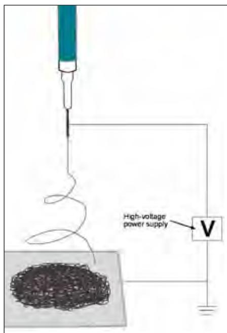
**Fig. 2:** Typical laboratory-scale electrospinning apparatus that allows production of milligram to gram amounts of ceramic nanofibers.
