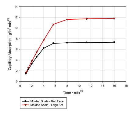
For molded brick, we do not see as much difference between the orientation directions.
