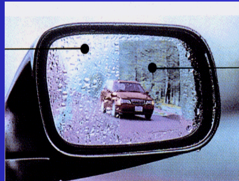
Right half of mirror only coated with photocatalytic film.
