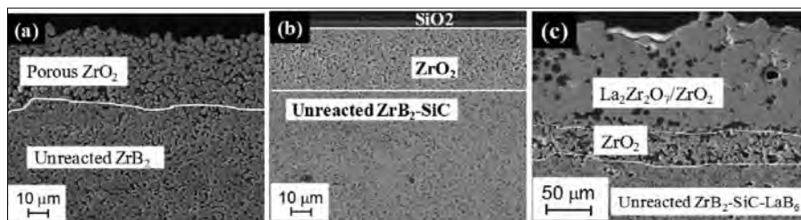
Figure 5 Cross-section microstructures of (a) ZrB_2 , (b) ZS20 and (c) ZS20- LaB_6 oxidized for 1 hour at 1600°C.
