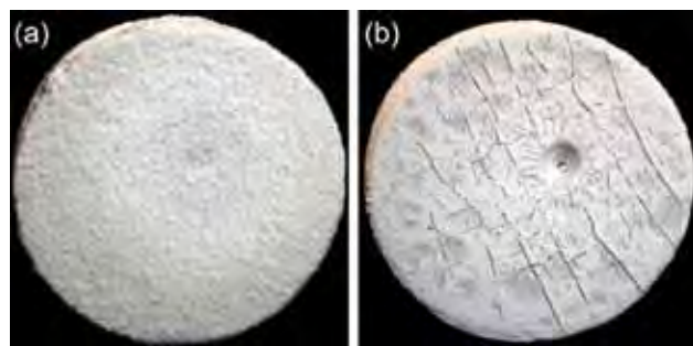
Figure 15 Carbon-fiber-HfB 2 composites after oxyacetylene torch testing after (a) 60 seconds showing negligible erosion and (b) 140 seconds showing less than 2-millimeter erosion.
