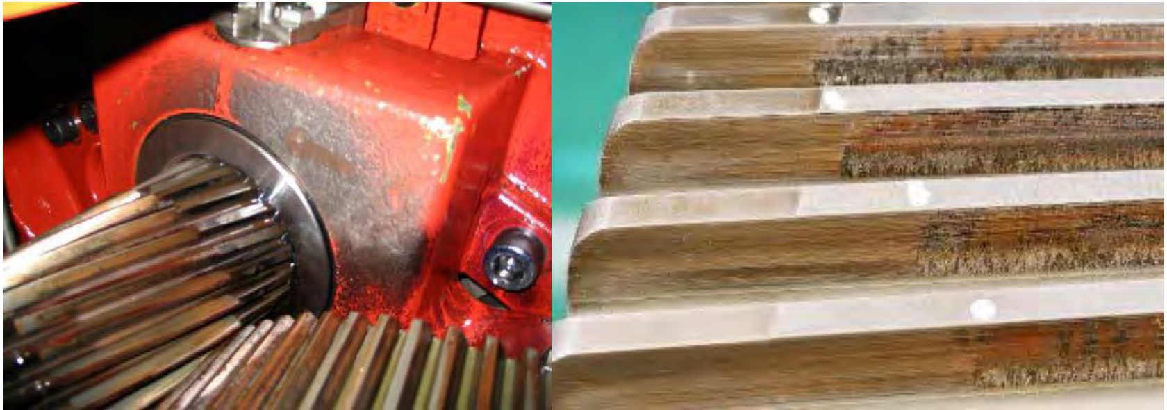
GRC Gearbox 1 high-speed stage displaying damage.
