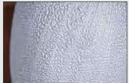
Artists and engineers usually try to avoid crawling of glazes (left), but an intentionally crawled glaze can enhance aesthetic appeal.
