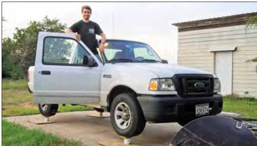
▲ John Mayo at Texas A&M used his truck to test the compressive strength of ordinary coffee mugs.
