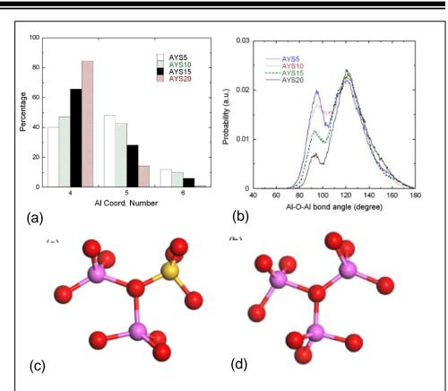
Fig. 1 (a) 4-coordinated Al increase and 5/6 coordinated Al decrease as SiO<sub>2</sub> concentration increases in aluminosilicate glasses from MD simulations. (c) and (d) snapshots of oxygen triclusters as a charge balancing mechanism in aluminosilicate glasses. Red ball: oxygen; organge ball: silicon; pink ball: aluminum.
