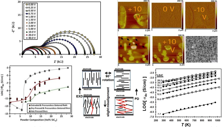
Properties of  $SiC_w$ - $Al_2O_3$  composites are anisotropic and depend on the processing,  $SiC_w$  content, interwhisker contact, electrodes, frequency, dc bias, and temperature.
