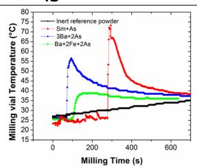
Build calorimeter to investigate thermodynamics of pnictide reactions
