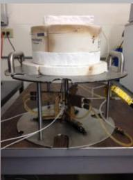
High temperature set-up for Resonant Ultrasound Spectroscopy developed and built at Texas A&M University.
