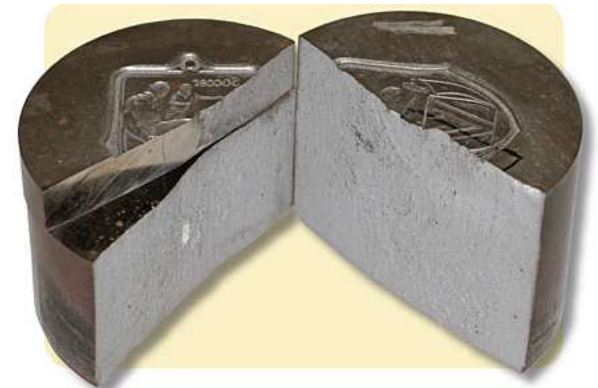
Steel quench crack
