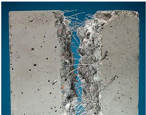
steel fiber reinforced concrete
