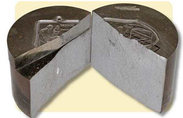
Steel quench crack
