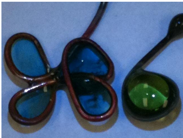
Figure 4. Borax beads formed with copper wire (blue bead) and nichrome wire (green bead)
