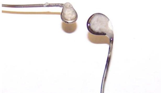
Figure 6. Beads that have a gray, milky color rather than a transparent, bright color due to the gas bubbles that remain trapped in the amorphous Borax
