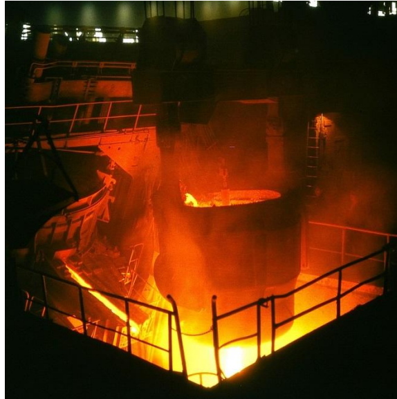
Figure 2. Steelmaking- refractory materials are used in the crucible.
