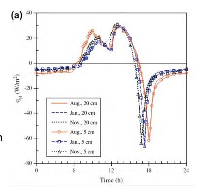
Figure 2: Energy Storage Rate for a Wall System [3]
