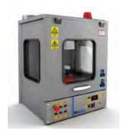
NE300 is the 40 kV model that allows you to do bottom to up electrospinning and nanofiber production on a plate collector and a D100mm X L220mm dimensioned max. 500 rpm rotating drum with multi-nozzles up to 9 in its electrically insulated chassis with 30-230 mm automatic spinning distance control&indicator (in mm.) and automatics options as LED
