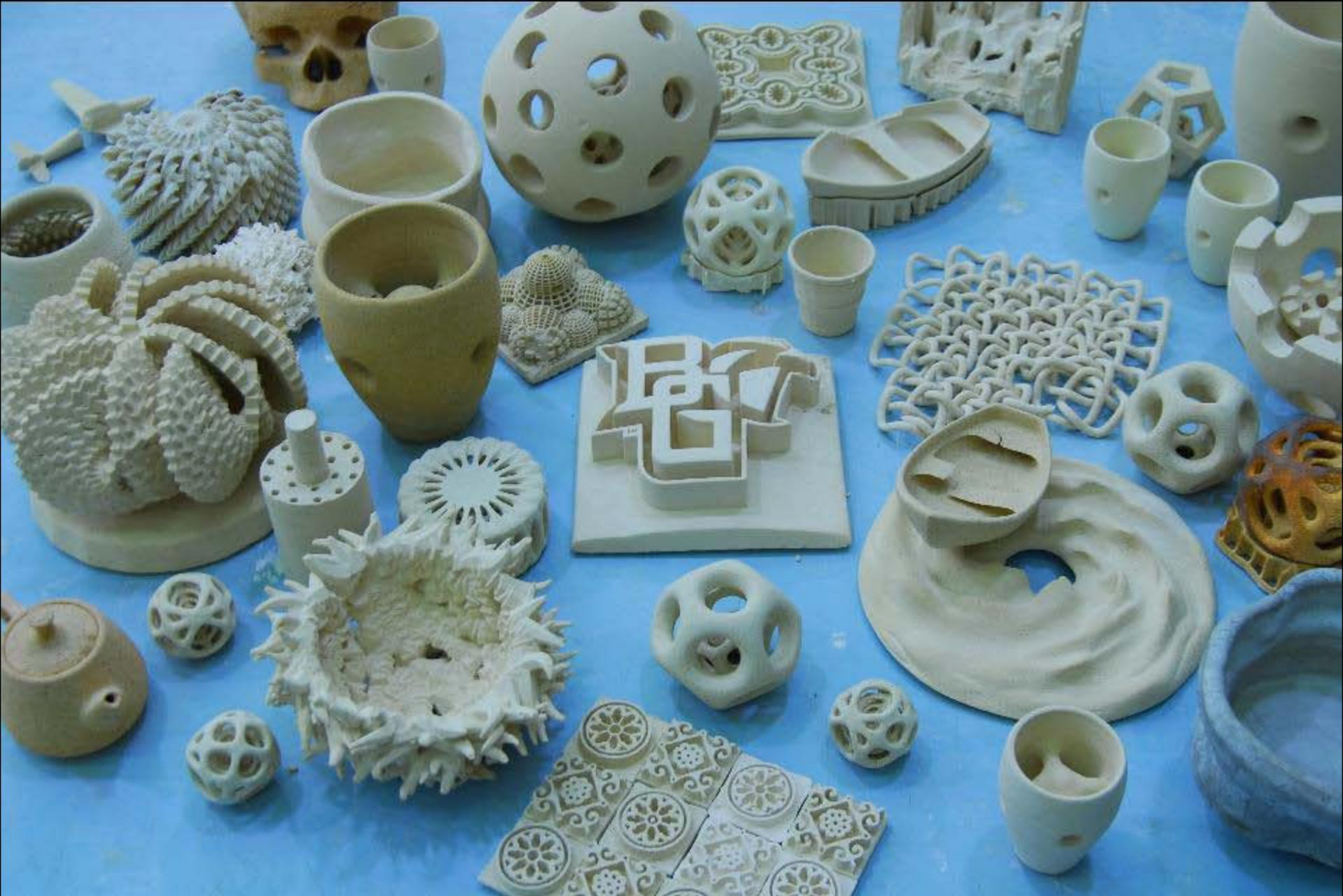
We have discovered a way to create ceramics by printing objects from a digital file using a rapid prototype machine.
