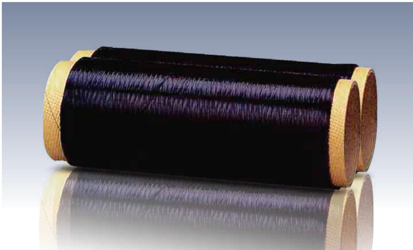
Developed using our unique technology, Tyranno Fiber® is a continuous ceramic fiber comprising of Si, Ti or Zr, C and O. Advanced composites reinforced by Tyranno Fiber are expected to play an important role in future environmental fields such as ultra high speed transportation, energy efficiency, CO<sub>2</sub> and NO<sub>x</sub> reduction, and purification of exhaust fumes.
