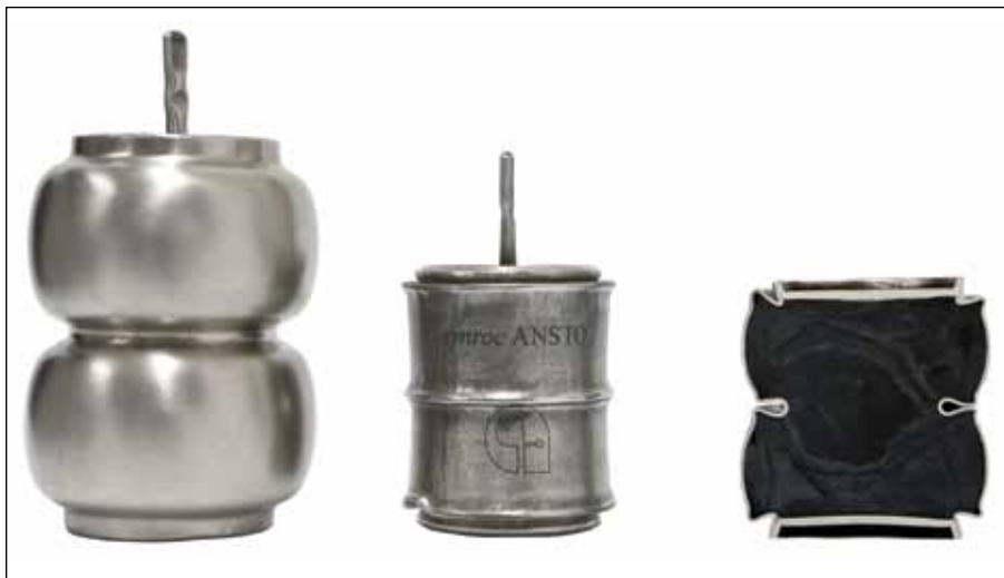
ANSTO's synroc hot isostatic pressing technology can reduce radioactive waste volume. Metal cans are loaded with radioactive nuclides and a ceramic powder, and then hot isostatically pressed to encapsulate solid waste for disposal into a repository.
