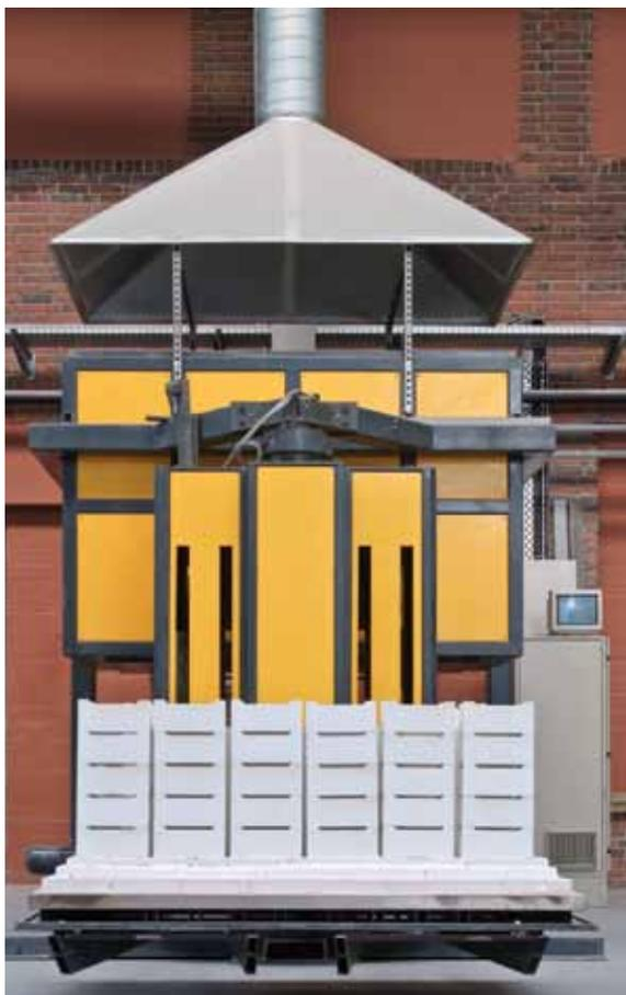
**Figure 3. Electrically heated top-hat kiln fires at temperatures up to 1,700°C.**
