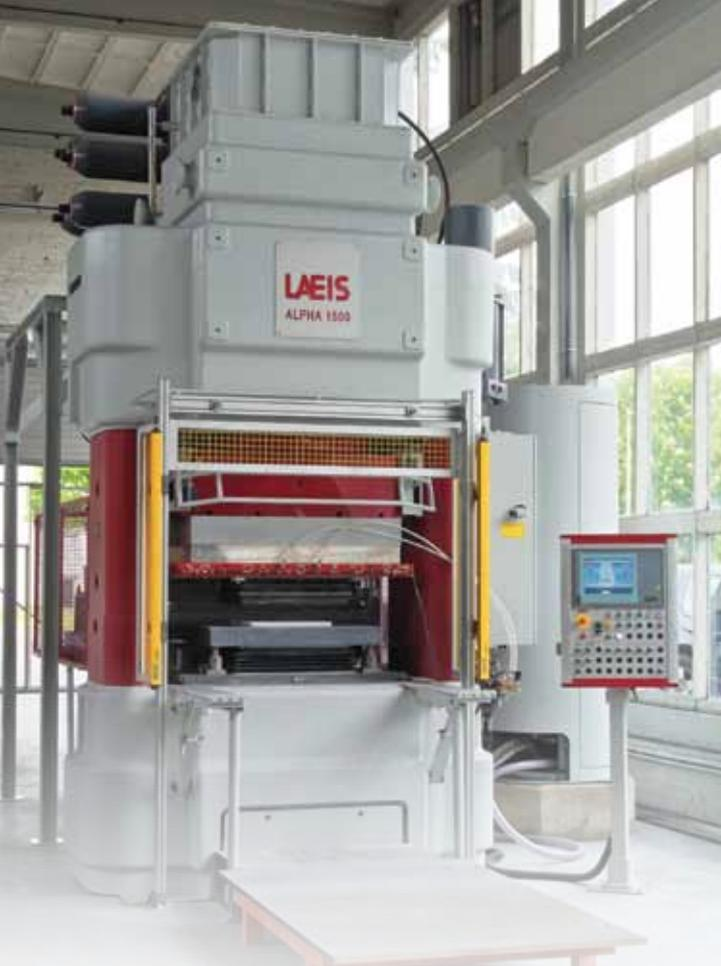
Figure 1. Hydraulic press Alpha 1500 with 1,500-ton pressing force and filling height of 120 mm.
