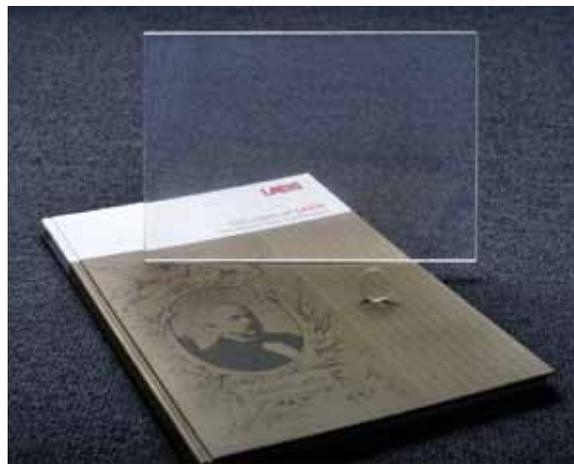
**Figure 6. Transparent spinel plate (220 x 300 mm x 4 mm).**
