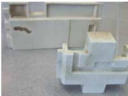
**Figure 5. Vacuum pressing eliminates structural defects in cordierite stacking aids with large height variations.**
