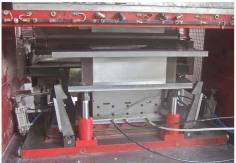
Figure 2. Mold for pressing saggars with more than 120 mm filling height in the Alpha 1500 press.
