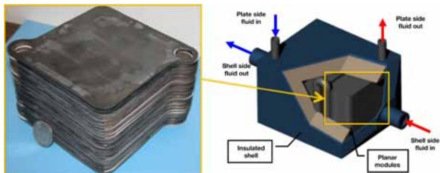
Figure 3. A stack of silicon carbide heat exchanger plates (left) and a conceptual design of modular, microchannel plate heat exchanger for a macroscale process (right).
