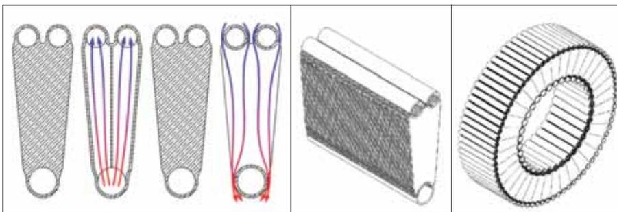
Figure 12. Design of a microchannel recuperator for a microturbine showing the microchannel architecture (left), a modular segment (middle), and the complete assembly.
