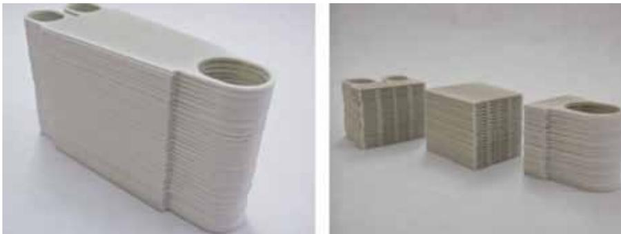
Figure 13. Segment of mullite microturbine recuperator fabricated at Ceramatec.
