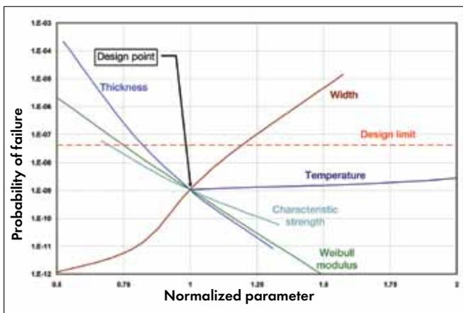
Figure 8. Sensitivity of microchannel reliability to design parameters.
