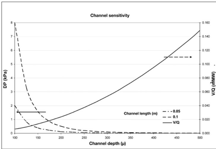
**Figure 4. Competing effect of channel depth and device performance, V/Q, on pressure drop.**
