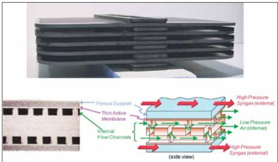
**Figure 14. Clockwise from bottom right: Conceptual design for ceramic catalytic membrane reactor for process intensification; cosintered microchannel structure detail; and a modular component for prototype testing.**
