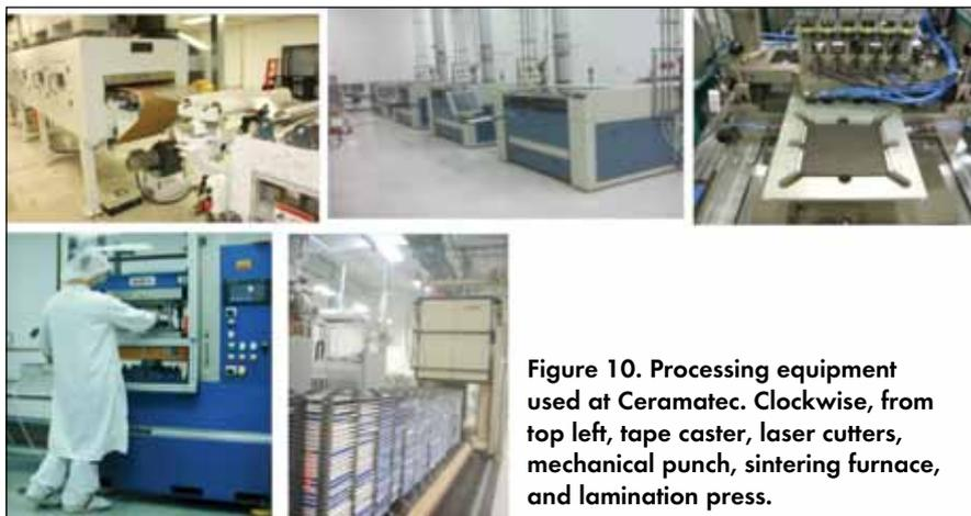
Figure 10. Processing equipment used at Ceramatec. Clockwise, from top left, tape caster, laser cutters, mechanical punch, sintering furnace, and lamination press.
