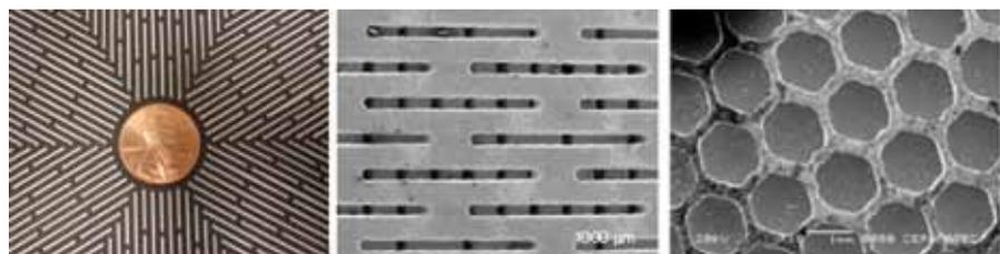
Figure 2. Examples of ceramic microchannel designs fabricated by Ceramtec showing a green layer (far left) and sintered layers (middle and right).
