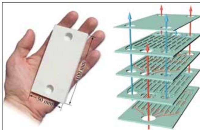
Figure 9. Alumina microchannel component made by dry-pressing and green-joining.
