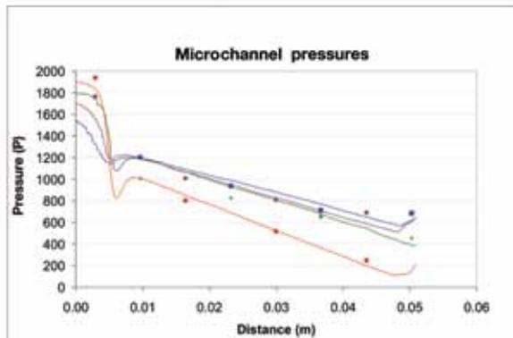
**Figure 5. Apparatus for measuring pressure in microchannel components (left), and comparison between measured (points) and computed (lines) pressure in a microchannel heat exchanger plate as a function of position (right).**
