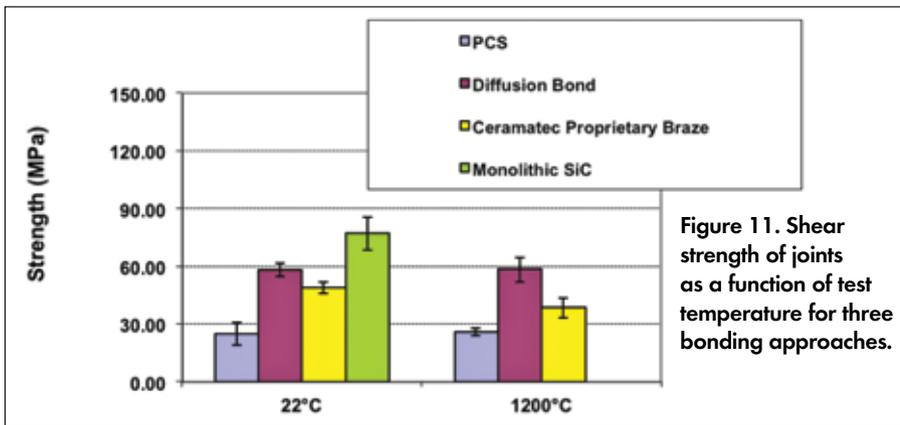
Figure 11. Shear strength of joints as a function of test temperature for three bonding approaches.
