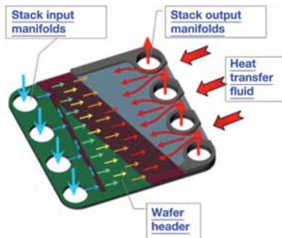
Figure 1. Schematic design of a microchannel plate for a ceramic heat exchanger.
