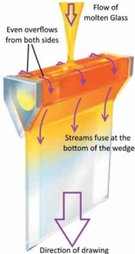
**Figure 2. Corning fusion overflow process for producing thin glass (adapted from corning.com).**
