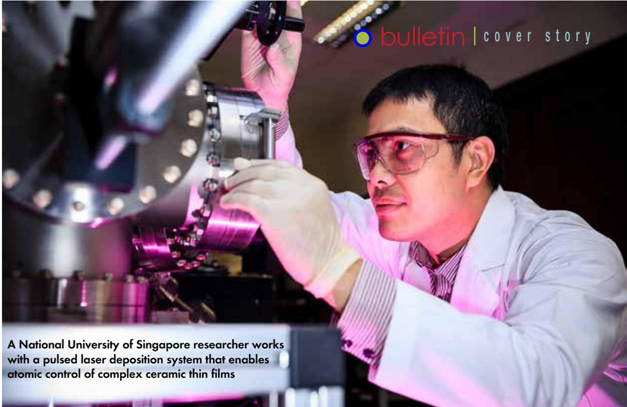
A National University of Singapore researcher works with a pulsed laser deposition system that enables atomic control of complex ceramic thin films
