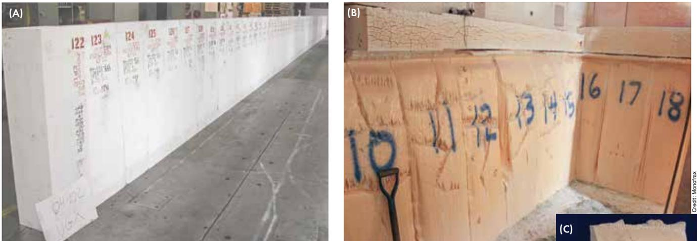
**Figure 1. (A) New AZS furnace lining during inspection before delivery and installation. (B) Corroded AZS furnace lining after 6.5 years of service in a soda-lime glass furnace. (C) Close-up of a corroded AZS furnace lining panel after 6.5 years of service in a soda-lime glass furnace.**
