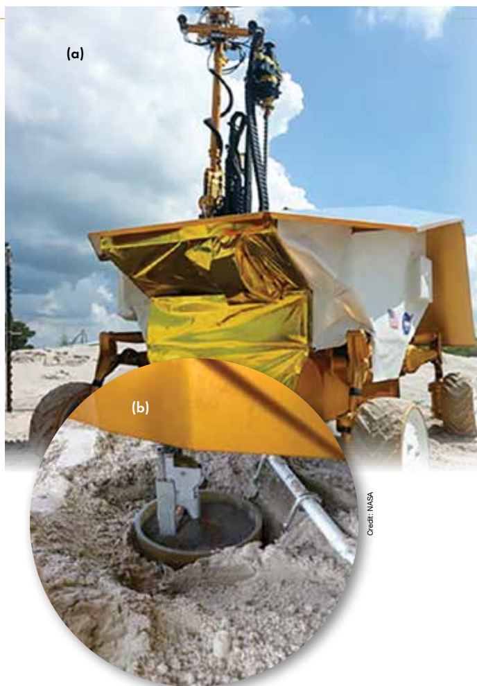
Figure 1. (a) NASA's Resource Prospector prototype utility vehicle in the rock yard of NASA Johnson Space Center. (b) Resource Prospector can drill into the ground to collect soil samples.
