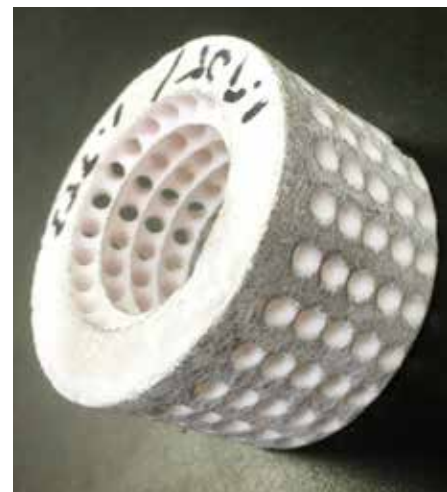
Figure 3. 3-D-printed ceramic object, with an outer diameter of ~5 cm, and height of ~3 cm.
