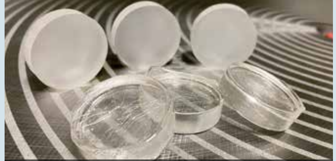
DCM Tech automated rotary surface grinders can be used to grind flat glass to precise dimensions before polishing, significantly reducing intermediate lapping steps as well as preventing breakage of what is often a high-value product. Above, glass discs before and after grinding. Credit: DCM Tech
