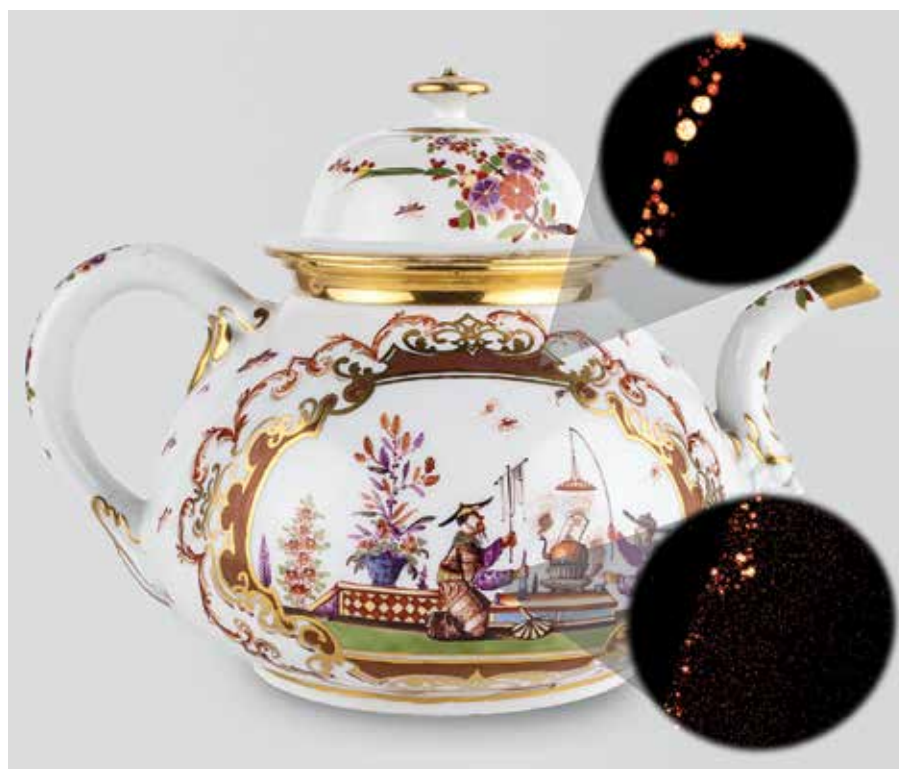
18 th century Meissen teapot (Art Institute of Chicago) with Böttger luster (top) and Purple of Cassius enamel (bottom) noted with cross-sectional maps of gold nanoparticle signatures from energy dispersive X-ray spectroscopy.
