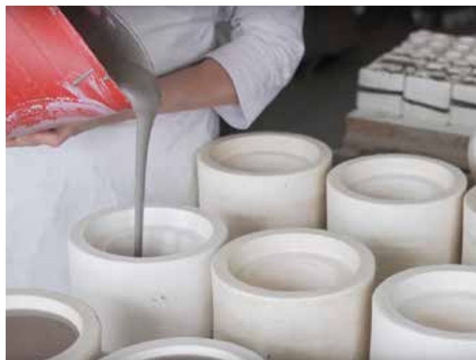
Example of slip casting a ceramic mug. A new study found forming method influences the microstructure of flash-sintered ceramics.
