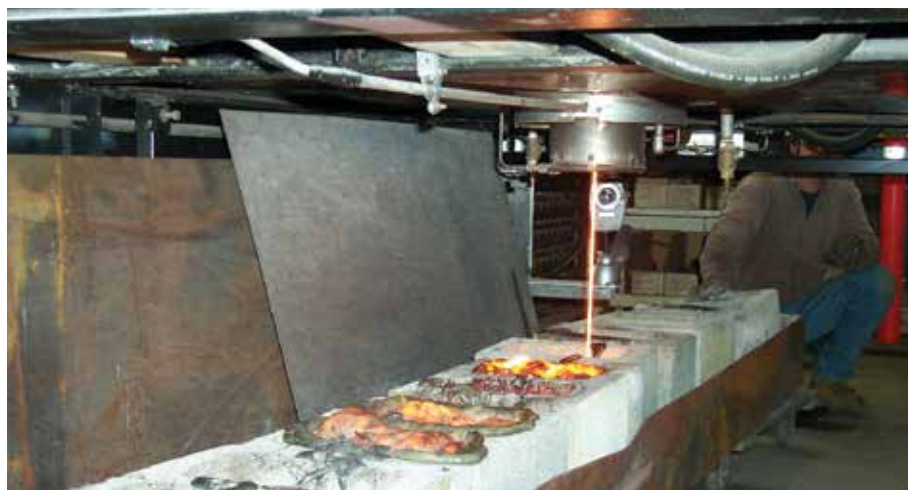
Fig. 2. Melt drops out the bottom-pour electric furnace into collection pots.
