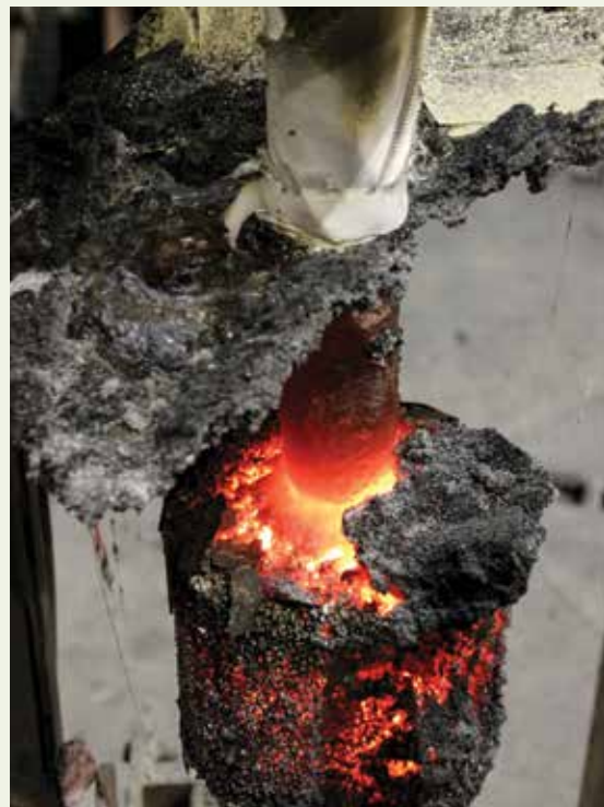
Figure 1. Carbon-bonded alumina filter after application in the industrial tundish.
