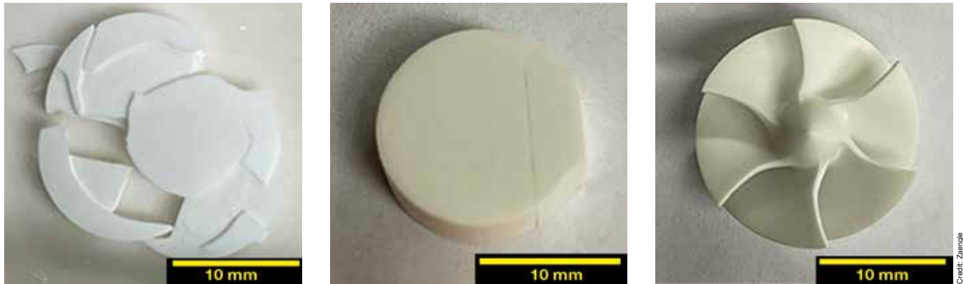
Figure 1. Tosoh TZ-8YS sintered samples, printed from slurry with 42.5% solid loading. Left and center show two common failures (cracking and flaking) and right shows a sample with complex geometry that sintered successfully.
