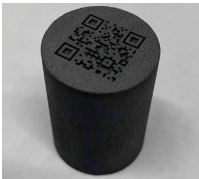
Figure 4. 3D-printed SiC part at Ultra Safe Nuclear with unique tracking ID.
