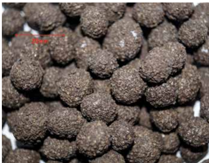
Figure 2. Kraftblock heat storage granules.
