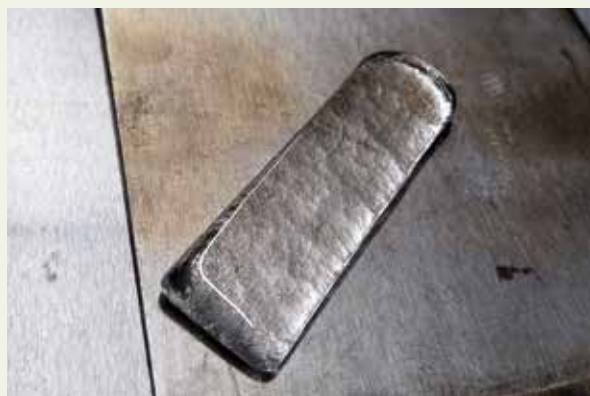
Figure 1. Bar of LionGlass made at The Pennsylvania State University for mechanical testing.
