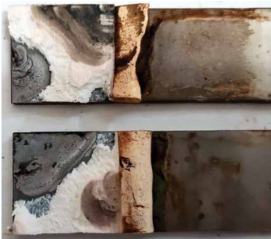
Corrosion observed deep in the bondlines of 316 steel metal-metal lap shear specimens conditioned at Pacific Northwest National Laboratory.
