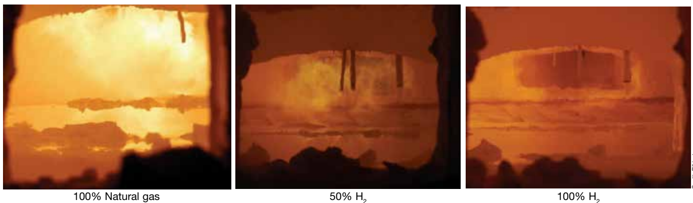
Figure 2. Glass melting trial in a flat glass furnace using a single port burner showed glass melting in progressively hydrogen-rich fuel mixes starting with 100% natural gas, 50% each natural gas and hydrogen, and 100% hydrogen.
