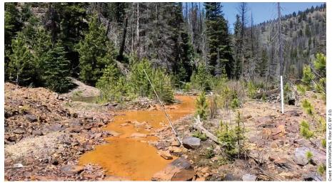
Acid mine drainage from the Mike Horse Mine complex in Montana. Acid drainage is often marked by "yellow boy," a yellowish-orange substance that occurs when the pH of acidic mine drainage rises above pH 3, so that the previously dissolved iron precipitates out.
