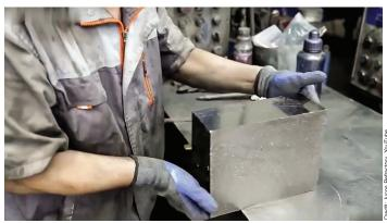
A worker handles a magnesia carbon brick at a Zibo Jucos Co., Ltd. plant in China. MgO–C bricks can be fabricated using various carbon sources, and significant effort has gone into determining which source can best improve the brick's thermal shock resistance.
