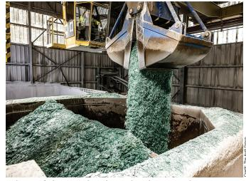
Delivery of glass recyclate during the GlassLoop pilot project, which explored the potential of recycling defective car glass back into new windshields.
