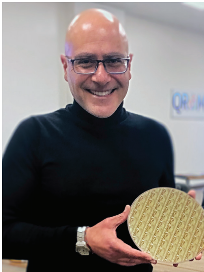
Cem Basceri, QROMIS president and CEO, displays a 200-mm-diameter 650 V, E-mode gallium nitride discrete power device wafer on a QROMIS Substrate Technology (QST®) substrate.
