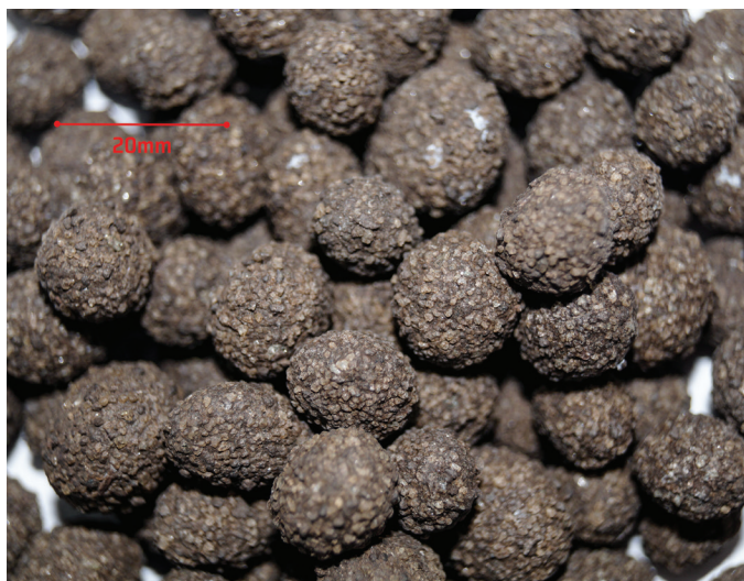
Figure 2. Kraftblock heat storage granules.
