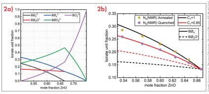
Figure 2. (a) Theoretical fraction of short-range order structural units in binary zinc borate glasses with the fictive temperature-dependent constant set to 1. Note that beyond x=0.667 the fractions of metaborate triangles and tetrahedra are identical. (b) Comparison of theoretical and experimental (B<sub>4</sub> only) fraction of metaborate type species in the bulk glass-forming range; NMR data by R. Youngman, Corning.
