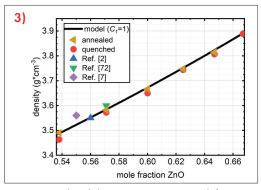
Figure 3. Predicted density using SROCM with fictive temperature dependent constant set to 1 compared to experimental values for binary zinc borate glasses measured in this study (orange triangles and red circles) along with several literature values.
