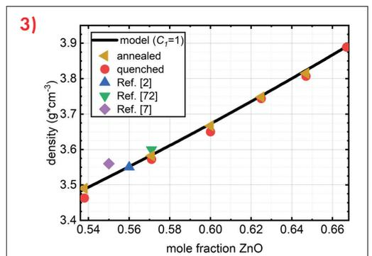
**Figure 3.** Predicted density using SROC model with fictive temperature dependent constant set to 1 compared to experimental values for binary zinc borate glasses measured in this study (orange triangles and red circles) along with several literature values.
