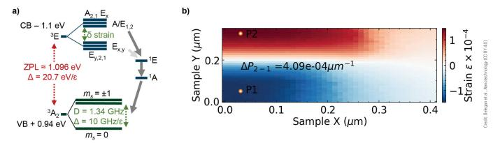
Figure 2. a) Energy level diagram of VV° defects in 4H-SiC as a function of strain relative to the conduction band (CB) and valence band (VB). b) At about 10 nm step size in a high-resolution raster nanodiffraction scan of a screw-dislocation running in-plane, we note a drastic change in strain from tensile to compressive, showing a 1.14 × 10<sup>-4</sup> variation in strain over 0.28 µm. P1 and P2 are theoretically plausible locations for two VV° defects within the same optical spot-size.
