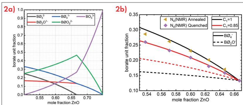
**Figure 2.** (a) Theoretical fraction of short-range order structural units in binary zinc borate glasses with the fictive temperature-dependent constant set to 1. Note that beyond  $x=0.667$  the fractions of metaborate triangles and tetrahedra are identical. (b) Comparison of theoretical and experimental ( $B_4$  only) fraction of metaborate type species in the bulk glass-forming range; NMR data by R. Youngman, Corning.
