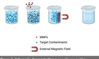
Figure 1. Schematic demonstrating magnetic separation. Contaminating blue particles are sorbed by magnetic red particles and then separated out using an applied magnetic field.
