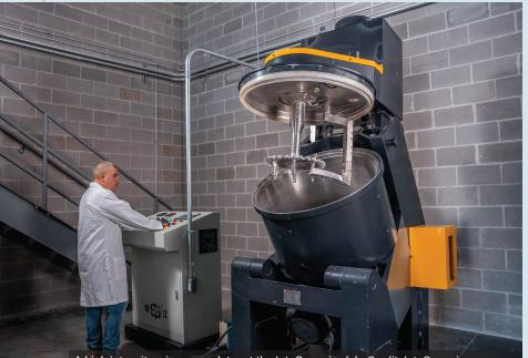
A high intensity mixer-granulator at the IntoCeramics lab. Credit: IntoCeramics
