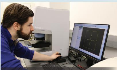
Arron Potter, postdoctoral researcher at the Center for Glass Innovation in Alfred University's Inamori School of Engineering, uses an infrared microscope on a fragment of glass taken from a wine bottle to measure the extent of damage caused to the bottle's interior surface by exposure to liquid. *Credit: Alfred University*
