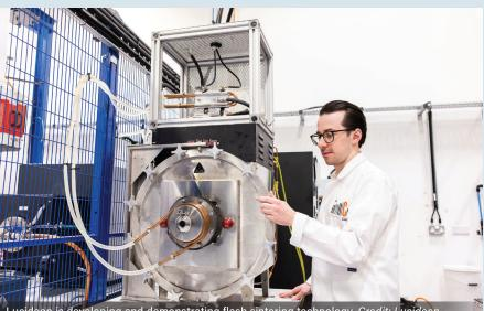
cideon is developing and demonstrating flash sintering technology. Credit: Lucideon
