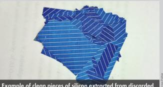
Example of clean pieces of silicon extracted from discarded solar panels using thermal delamination.
