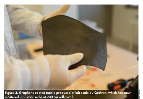
homogeneous, precise, and durable graphene coating of individual textile fibers. And the process can be applied to natural fibers like cotton, synthetic fibers like polyamide, and even glass and carbon fibers.
